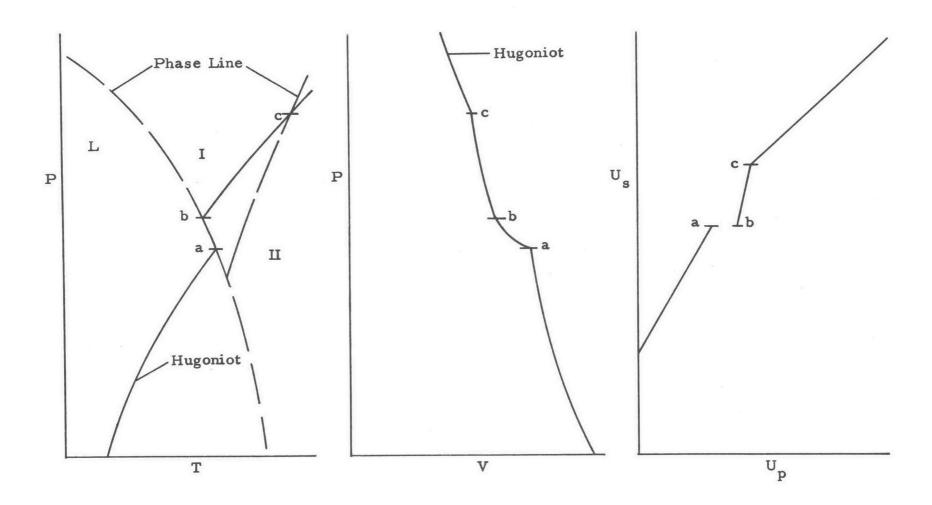
Fig. 24. Hugoniot passing through three phases.
